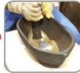
Au-Hg Amalgamation in process
