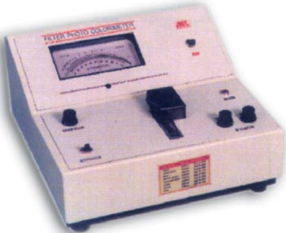
FIGURE 45.1: Photoelectric colorimeter used for taking reading of haemoglobin in cyanmet Hb method and oxyhaemoglobin method. (Photograph courtesy of Max Electronics India, Chandigarh).
