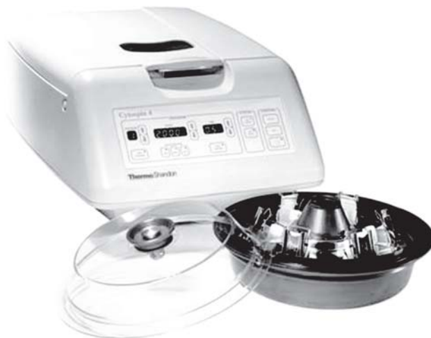
FIGURE 42.2: Cytospin used for making smears in cases with small volume of fluid (Photograph courtesy of Thermo Shandon, UK through Towa Optics India Pvt. Ltd., Delhi).
