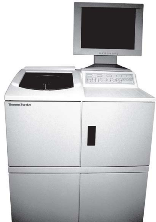
FIGURE 2.2: Vacuum tissue processor, Model Excelsior (Photograph courtesy of Thermo Shandon, UK through Labindia Instruments Pvt. Ltd., Delhi).
